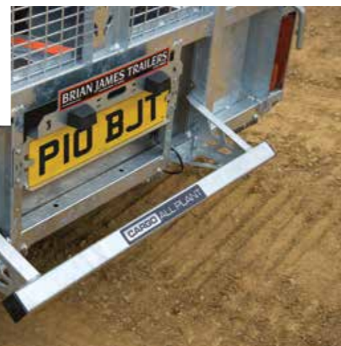
Easy ramp operation with gas spring assistance, enables opening and closing with less effort.
