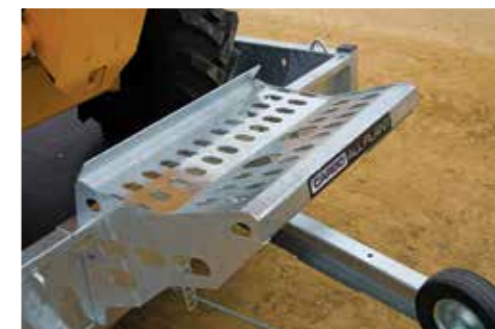
○ Purpose designed bucket rest is ideally located for digger buckets.
